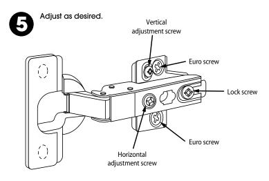
GAP ADJUSTMENT: Loosen lock screw, adjust gap by turning horizontal screw, tighten lock screw.
