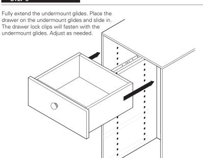
Drawer clips have integrated height adjustment to aid in alignment.
