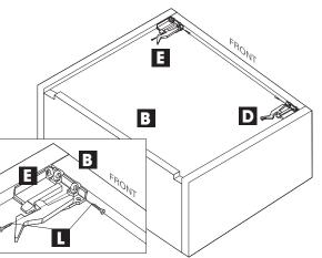
Attach the Drawer Glides (C) to the Vertical Panels with (4) Euro Screws (J) for the 14" Drawer Kits. For the 19" Drawer Kits attached with (6) Euro Screws (J). Add (2) additional screws, #7 x ½" Wood Screw, (I) in glide location shown. *Note: Extending the glides aids in accessing the hole locations.*
